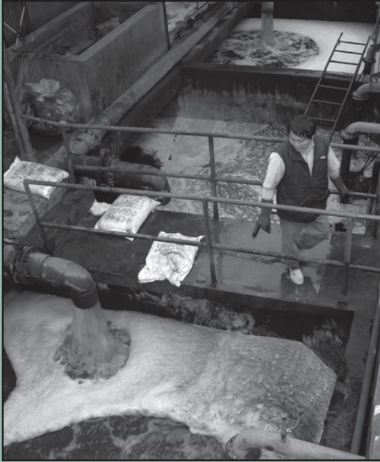
Aeration and biological treatment at a wastewater treatment plant in Guangdong Province. Photo Credit: Business for Social Responsibility
