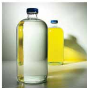
Amyris diesel fuel (clear) in front; petroleum diesel (yellow) in the back
